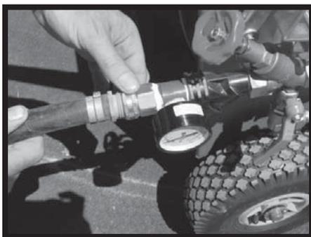
**IMPORTANT:** MAKE SURE SUPPLY HOSE IS CLEAN AND FREE OF FOREIGN OBJECTS THAT WOULD PLUG THE TURBINE SYSTEM OR SHUT OFF VALVE! INLET CONNECTION IS FITTED WITH A DEBRIS STRAINER THAT MAY NEED TO BE CHECKED FROM TIME TO TIME AND CLEANED IF FOREIGN OBJECTS OR MATERIAL ARE PRESENT IN INCOMING WATER.
